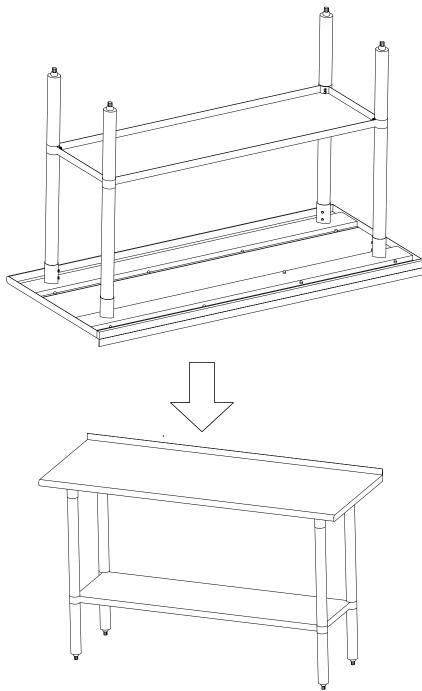
1. Turn the workbench over and remove the protect film on SS Top(A)and Adjustable shelf(B)
